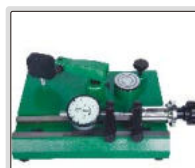
inspect accuracy of dial indicators (range 0-25mm)
